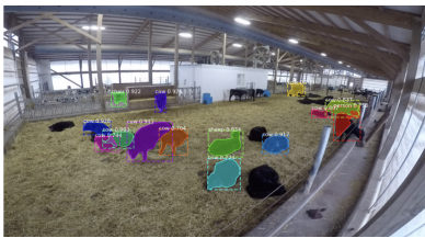
Figure 9. segmentation done on Angus cows using Mask RCNN
