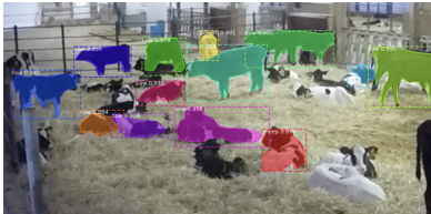
Figure 8. segmentation done on cropped image with cows in the back of the pen using Mask RCNN
